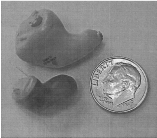
FIGURE 2. ITC (top) and CIC (bottom) self-contained ear-level device models to inhibit stuttering beside an American dime.
