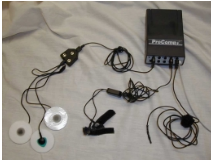
Figure 3.2. Procomp+ device. From left to right: the electrocardiograph, skin conductance, and skin temperature sensors.
