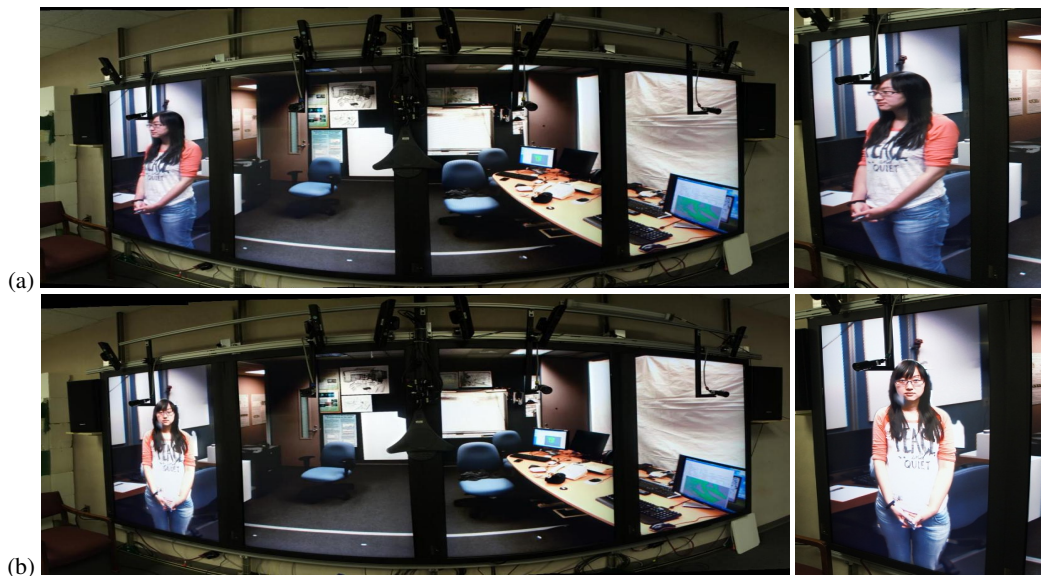
Figure 5: Comparison between the panoramic view and synthesized view of the camera switching algorithm. (a) the panoramic view with a side-facing person; (b) the synthesized view with the panoramic background and the front-facing person.
