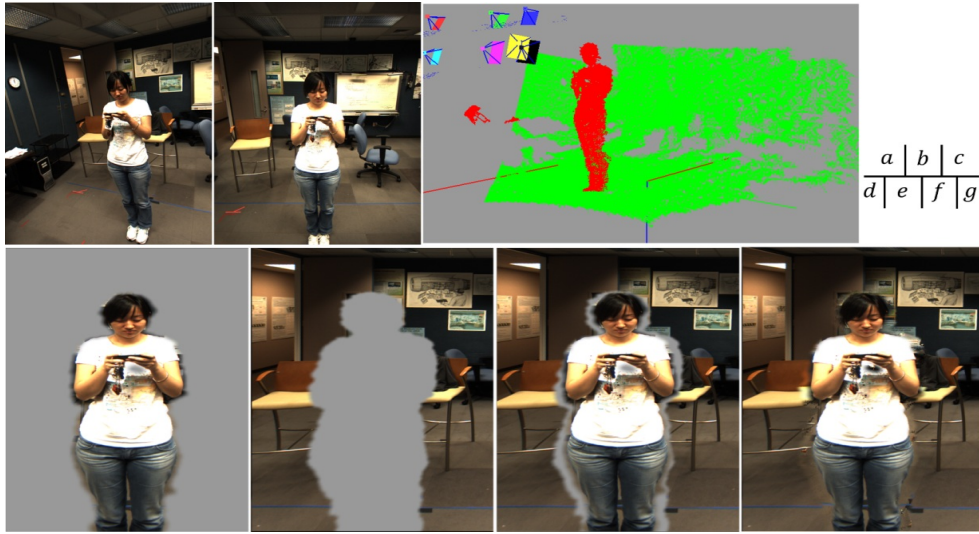
Figure 4: Various Intermediate results for one display panel during the operation of the system. (a) the image from one panorama camera after correcting lens distortion; (b) the image from one personal camera; (c) the foreground point cloud and background point cloud from depth sensors after performing segmentation; (d) the segmented foreground in the personal camera; (e) the segmented background in the panorama camera; (f) merge (d) and (e); (g) the synthesized image after hole filling.
