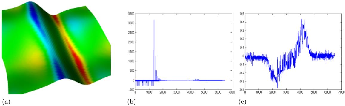
Figure 2: A 3D surface that has locally nearly flat regions with slight additive noise Fig. 2(a), with smoothed regularized curvature estimate as colormap. A direct least-squares paraboloid fit leads to unstable per-vertex curvature estimates Fig. 2(b) that are beyond repair by mesh averaging. Our regularized curvature estimation creates curvature estimates that are quite useable for geometric techniques after a smoothing filter Fig. 2(c)
