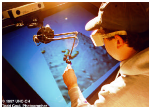
Figure 1: Physics Graduate Student Scott Paulson uses the nanoManipulator to examine a tobacco-mosaic virus particle.
