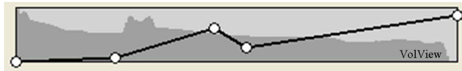
Figure 3.8: Example scalar opacity transfer function showing control points, piece-wise linear function, and a histogram of the data values.
