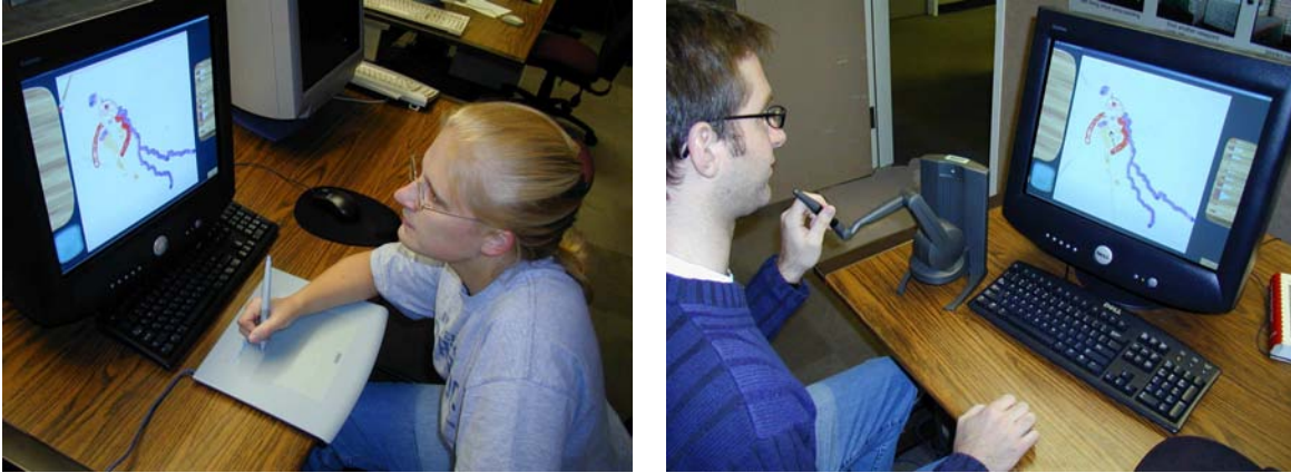
Figure 2.1: In my system, user input is obtained either through a 5-DOF Wacom TM tablet (left) or a 6-DOF Phantom TM haptic interface (right).
