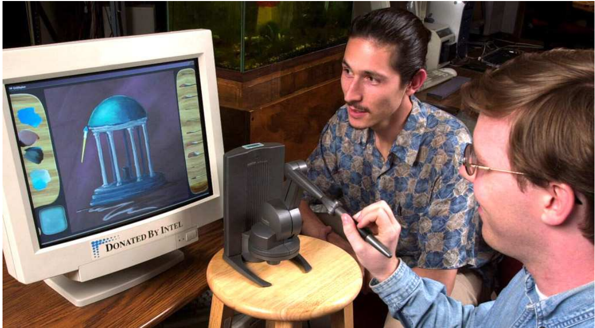
Figure 1.10: Artists paint by manipulating an input device, like the haptic stylus shown above, to control a 3D virtual paint brush. The results are displayed interactively and continuously as the artist works.
