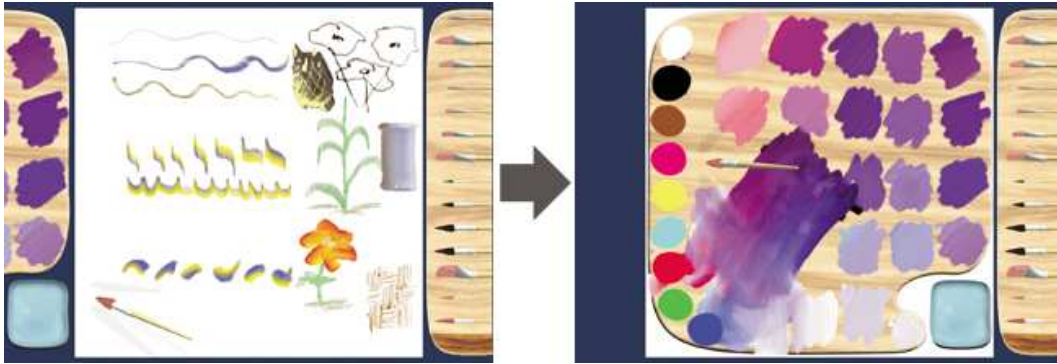
Figure 8.1: Graphical User Interface: The virtual canvas with the brush rack and a portion of the palette (LEFT); the brush rack and the palette for color mixing (RIGHT).
