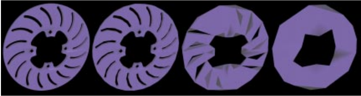
Figure 3.14: The original Rotor object and its LODs created by GAPS. From left to right these LODs consist of 4,736 faces, 1,184 faces, 296 faces, and 72 faces.
