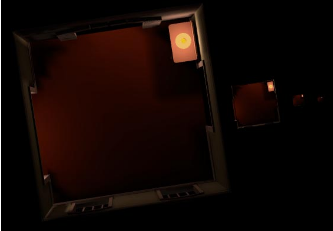
Figure 3.21: Switching distances for LODs of the Chamber object if we allow 1 pixel of error. From left to right these LODs consist of 7,817 faces, 5,211 faces, 2,605 faces, and 1,302 faces. The original object consists of 10,423 faces.
