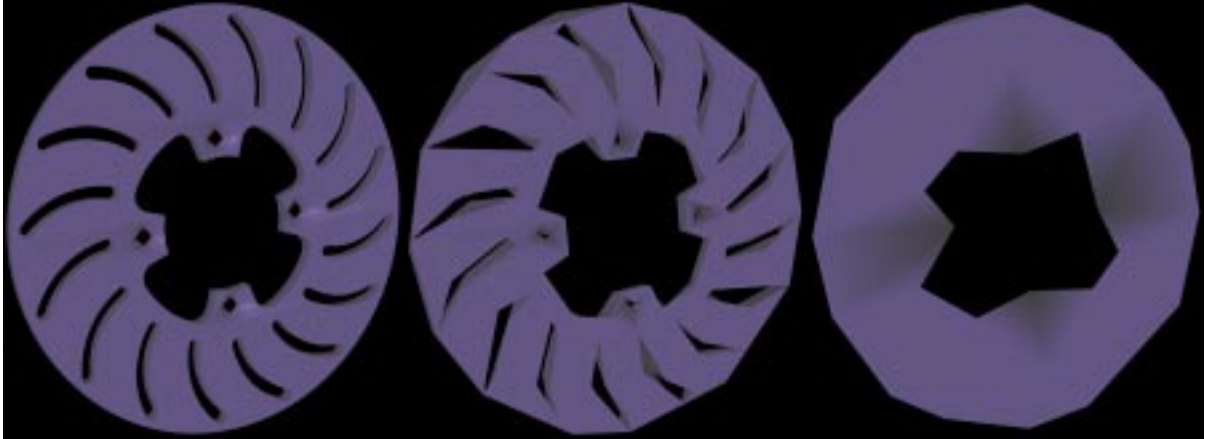
Figure 1.7: The benefits of topological simplification. The original Rotor model, consisting of 4,735 polygons, is on the left. If we do not allow topological simplification, then we cannot eliminate the tiny holes in this object. The coarsest approximation we can produce without topological simplification is in the middle and consists of 480 polygons. On the right, we simplify the Rotor model's topology to produce a 68 polygon approximation.
