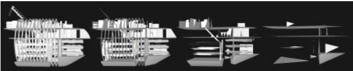
Figure 4.30: LODs created for the Torpedo Room model using the error quadric metric alone. They consist of 883,537 faces (the original model), 6,386 faces, 827 faces, and 100 faces.
