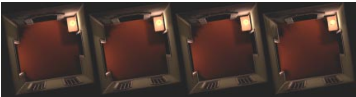
Figure 3.20: LODs for the Chamber object created by GAPS using the unified error metric described in Section 3.3.3.4. The results are superior to the LODs in Figure 3.19 in terms of color preservation. However, notice that the polygonal geometry of the lamp, i.e., the yellow ring, is preserved better in Figure 3.19. From left to right these LODs consist of 10,423 faces (the original object), 9,120 faces, 7,817 faces, and 5,211 faces.
