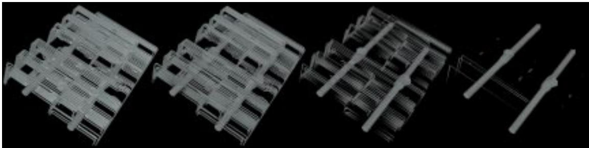
Figure 3.27: LODs for the ShDivWest object created by GAPS with no distance threshold and no surface area preservation. From left to right these LODs consist of 141,180 faces (the original object), 17,646 faces, 2,204 faces, and 272 faces.
