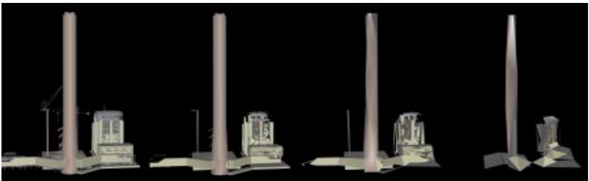
Figure 4.35: LODs and HLODs created for the Power Plant model using GAPS. They consist of 12,731,154 faces, 9,503 faces, 2,375 faces, and 590 faces.
