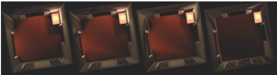
Figure 3.19: LODs for the Chamber object from a top-down view created by GAPS when error due to attributes is ignored. Note how the shadow and lighting information of this radiositized model rapidly disappears as the simplification proceeds. From left to right, these LODs consist of 10,423 faces (the original object), 9,119 faces, 7,817 faces, and 5,210 faces.
