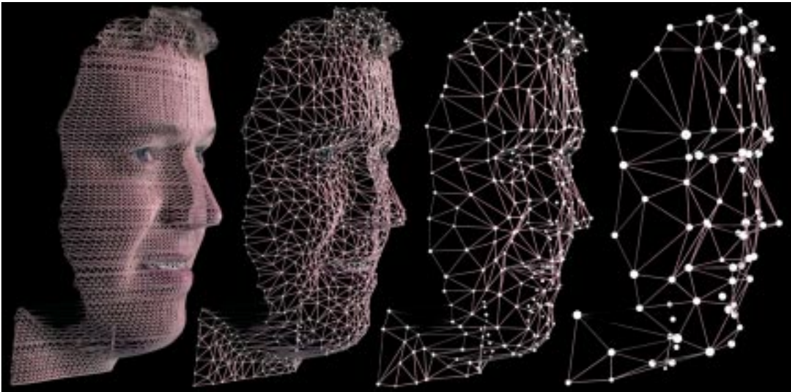
Figure 3.17: The approximate error bounds reported by GAPS for the same LODs as in Figure 3.16. The radii of the spheres are the approximate errors at the vertices they enclose as defined by the unified error metric in Section 3.3.3.4. These error bounds are used to automatically determine switching distances for LODs. From left to right these objects consist of 9,580 faces, 2,395 faces, 597 faces, and 148 faces.
