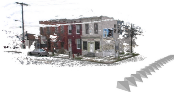
Figure 1: 3D-from-video: reconstructed 3D model including camera poses (shown as pyramids)
