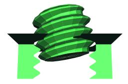
Figure 13: A cross-threaded bolt and nut configuration [NF91]
