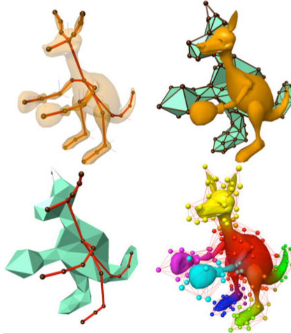
Figure 2.3: Local linearization. Capell et al. [CGC + 02a] associate each region of the finite element mesh with the bone of a simple skeleton and then locally linearize the elastic forces in the frame of that bone.
