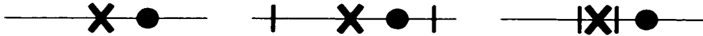
Figure 6.1: Floating-point guided computation. At left, a floating-point estimate (shown by the x) approximates the actual root (shown by the circle). At center, a bounding interval placed around the floating-point solution contains the actual root. At right, a smaller interval no longer contains the actual root.
