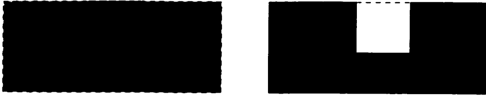
Figure 2.9: An overlapping face degeneracy. On the top, the solid to be removed shares a face with the solid being removed from. In a non-regularized operation, it is not clear whether the top face should or should not have a hole in it.
