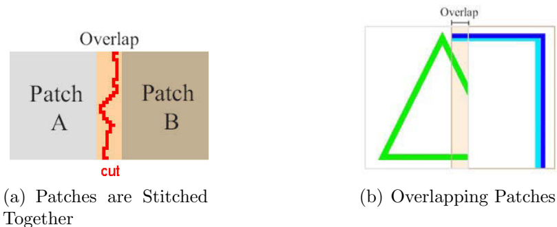
Figure 2.11: In patch-based texture synthesis, different patches are copied and overlapped slightly. A optimal cut is supposed to be made, but none of the cuts are good.
