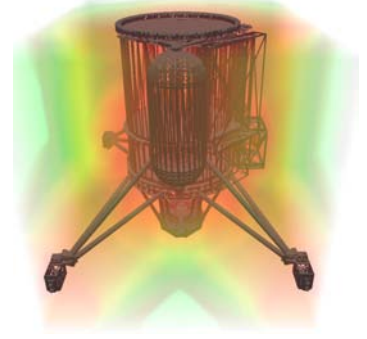
Figure 8. Cassini Model: A volume rendering of the distance field of the Cassini with 93K polygons. The distance to the surface is color coded, increasing from red to green to blue.
