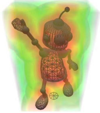
Figure 1. 3D Distance Field of Hugo Model(17k polygons): Distance to the surface is color coded, increasing from red to green to blue. Time taken to compute the distance field on 73 \times 45 \times 128 grid using our algorithm is 4.2 seconds.
